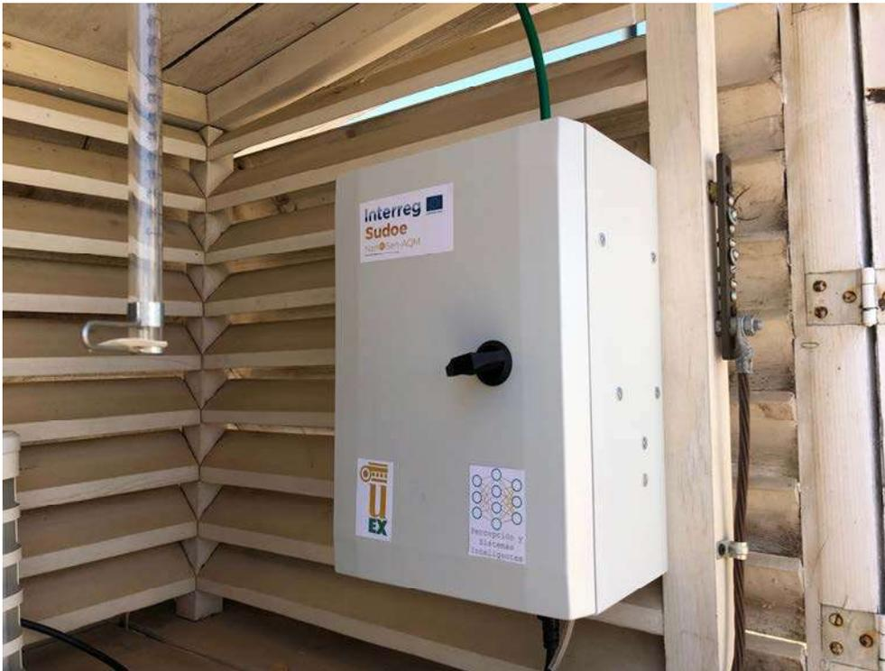
Figure 5: Air quality measurement system installed in parallel with the Badajoz reference station.
